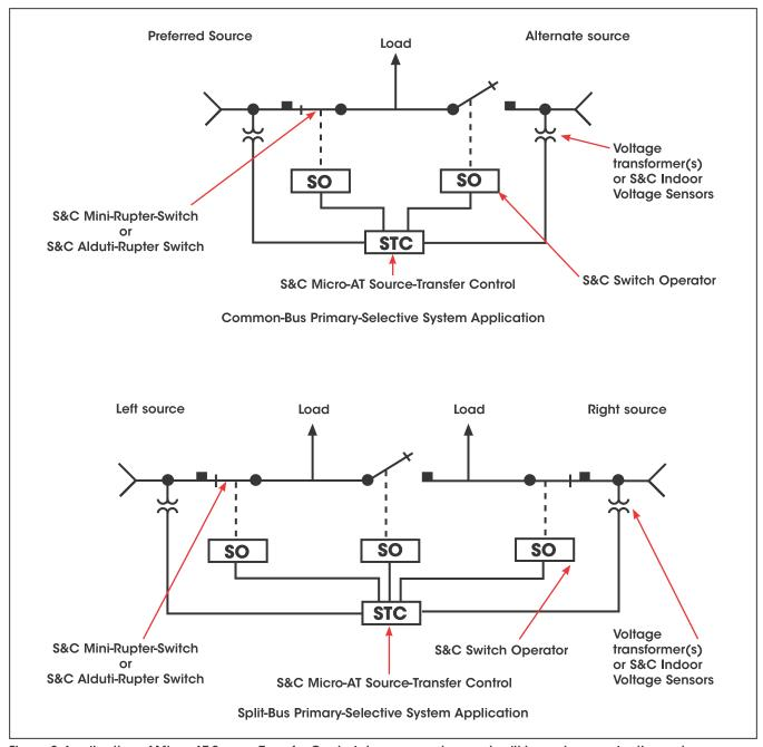
Figure 3.Application of Micro-AT Source-Transfer Controls in common-bus and split-bus primary-selective systems.
