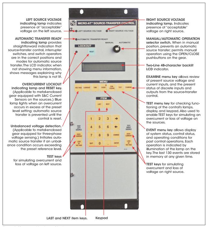
Figure 2. Close-up of front panel features.
