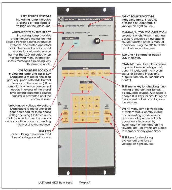
Figure 2. Close-up of front panel features.
