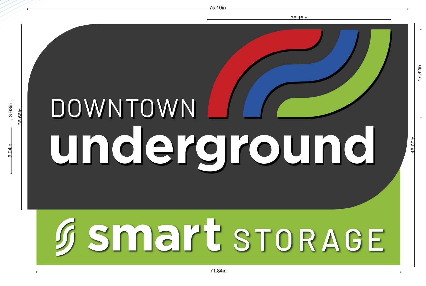
INTERNALLY LIT DOUBLE SIDED ROUTER CUT RADIUS CORNER CABINET 2" REVEAL ON LOWER PORTION
