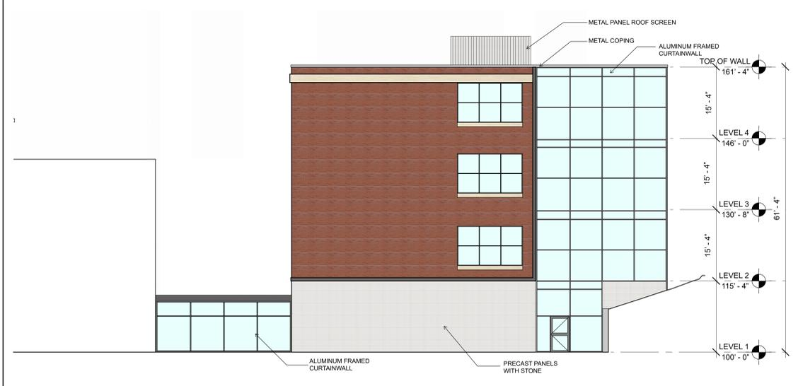
**F9** Scale 3/32" = 1'-0" Proposed Building B - Exterior Elevation - South
