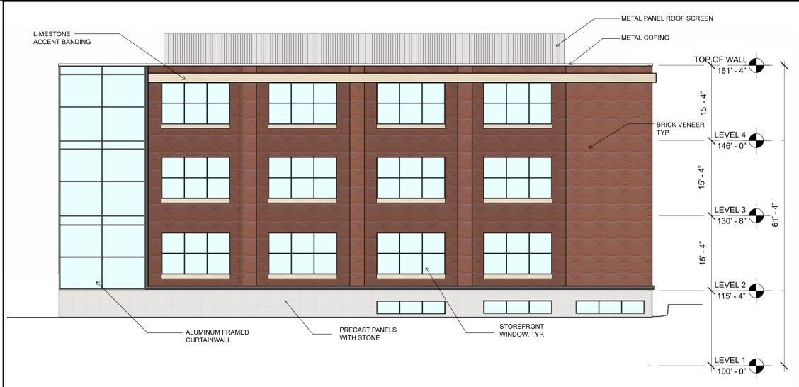
**A9** Scale 3/32" = 1'-0" Proposed Building B - Exterior Elevation - East
