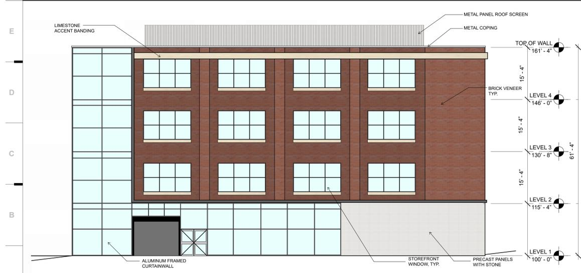
**A1** Scale 3/32" = 1'-0" Proposed Building B - Elevation West
