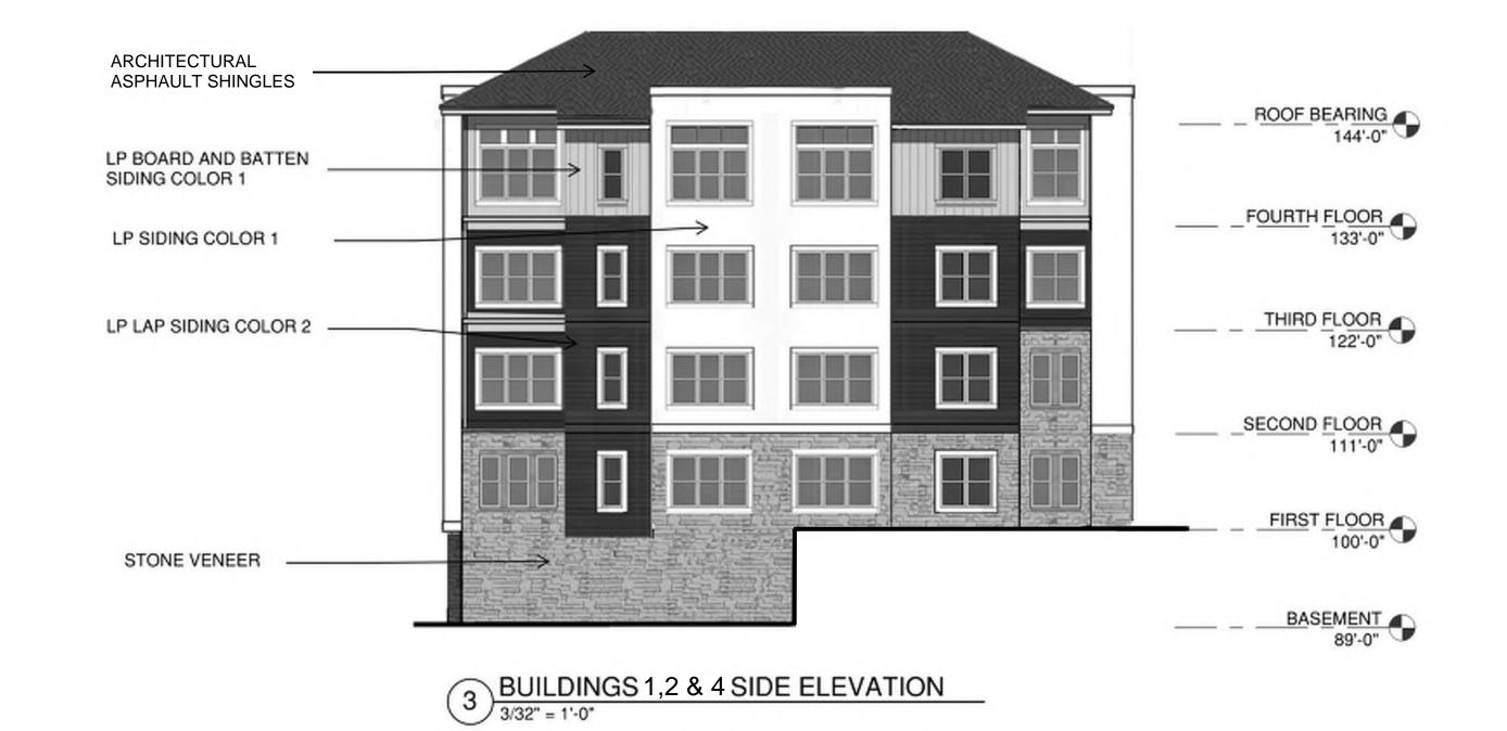
ARCHITECTURAL ASPHAULT SHINGLES ROOF BEARING 144'-0" LP SIDING COLOR 1 LP BOARD AND BATTEN FOURTH FLOOR SIDING COLOR 1 LP LAP SIDING COLOR 1 THIRD FLOOR LP LAP SIDING COLOR 2 PREFINISHED ALUMINUM **GUARDRAIL** SECOND FLOOR STONE VENEER
