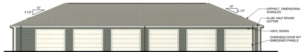
**2 ACCESSIBLE 6-BAY TYPE B, 6 STORAGE GARAGE FRONT ELEVATION**
