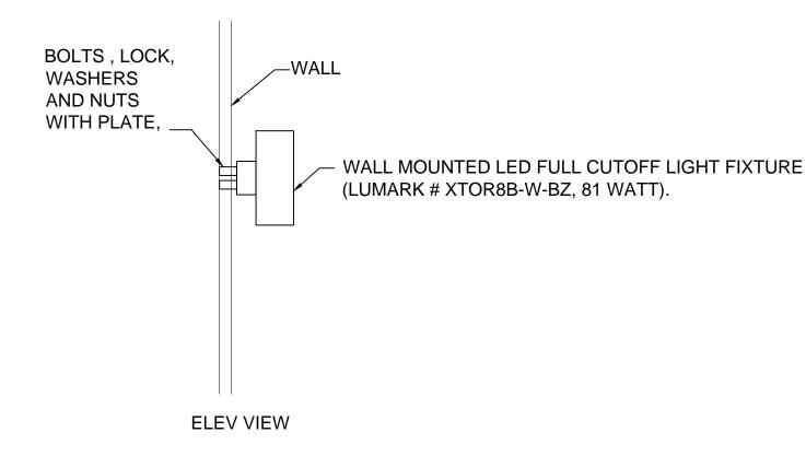
1 WALL MOUNT LIGHT FIXTURE TYPE 'W' DETAIL SCALE: NTS
