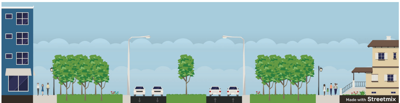
200-foot ROW: Two-way segment with wide median and park area between travel lanes and sidewalk
