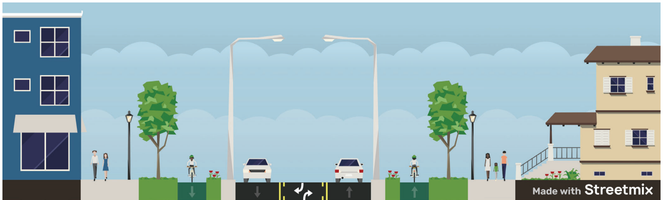
100-foot ROW: Two-way segment with center turn lane and separated mobility lane on both sides
