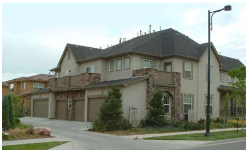
Provide residential dwelling designs with alternatives to street-oriented garages, such as a mixture of rear and side-loaded garages.
