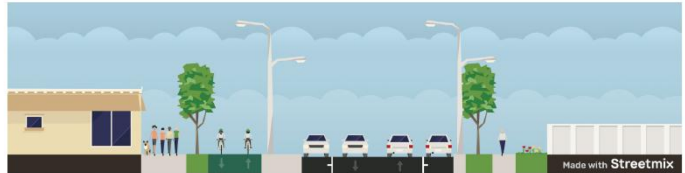
100-foot ROW: Two-way segment with parking lane on both sides and separated two-way mobility lanes
