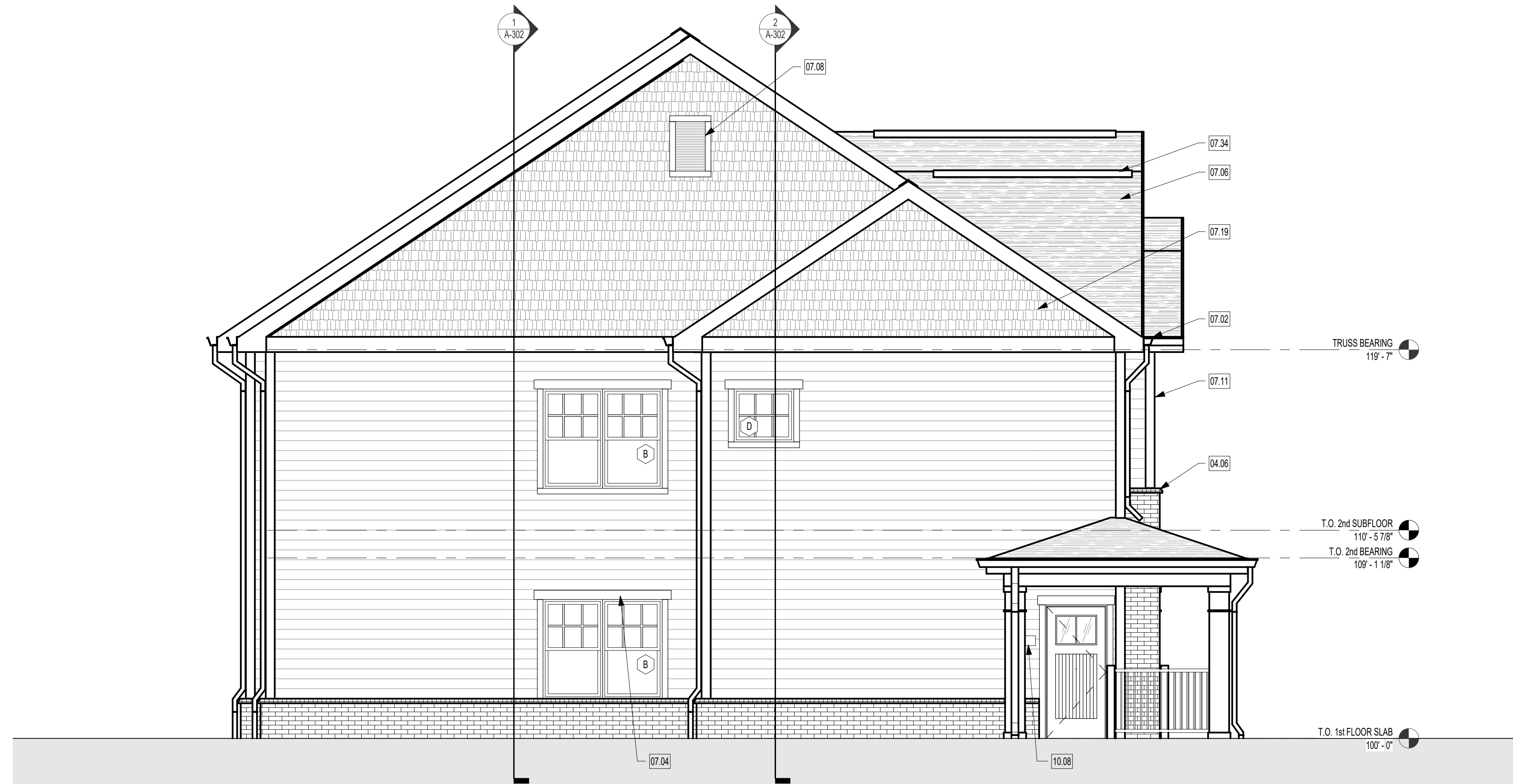
2 BLDG A - LEFT ELEVATION 1/4" = 1'-0"
