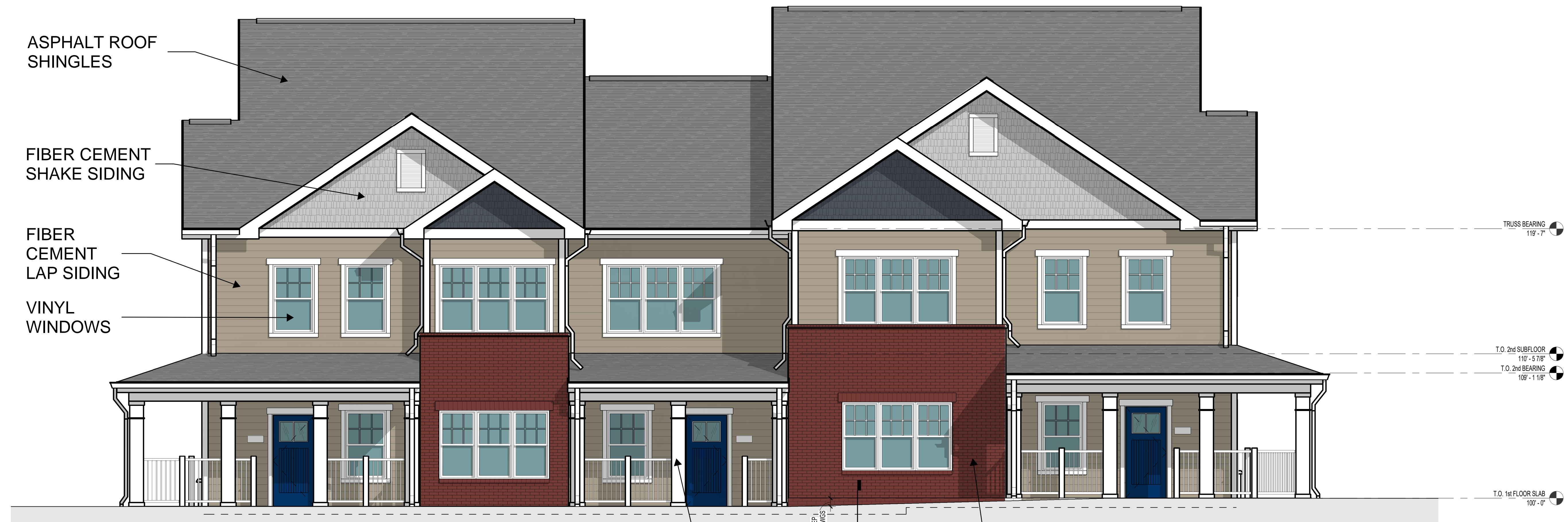
1 BLDG B #5 - STEPPED FRONT ELEVATION 1/4" = 1'-0"
