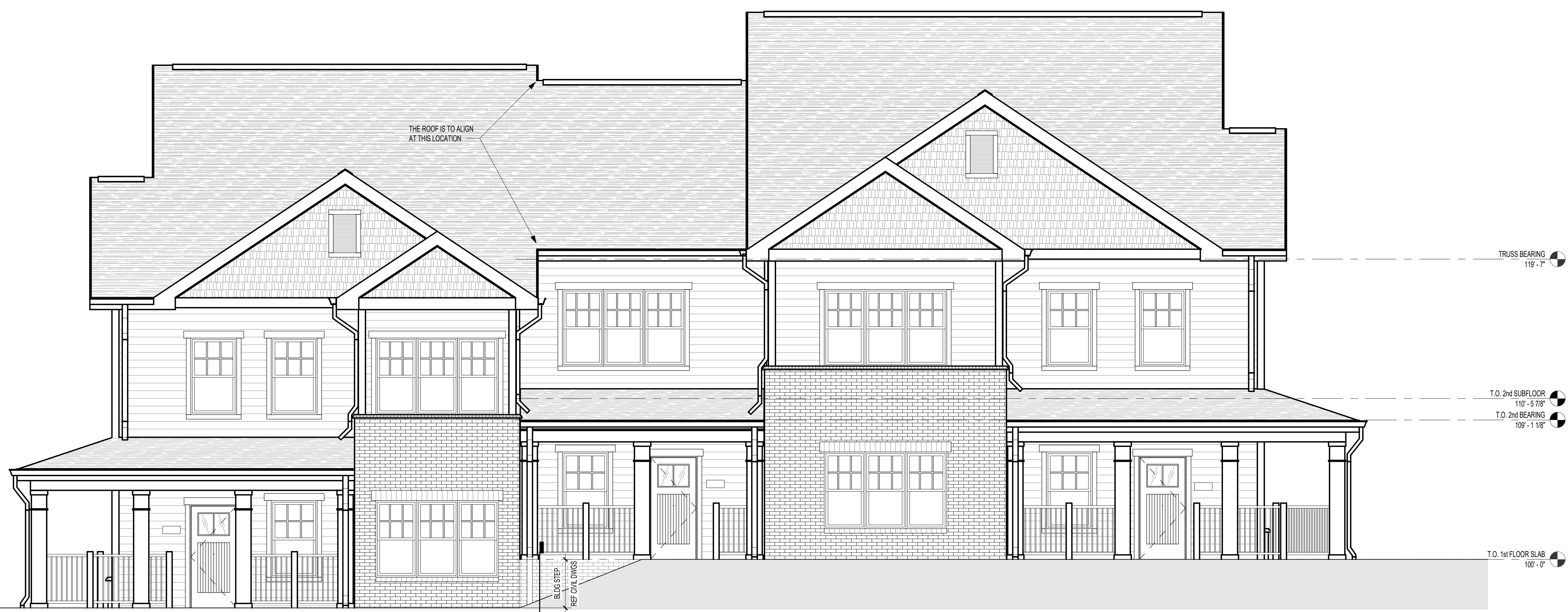
1 BLDG B #3 - STEPPED FRONT ELEVATION 1/4" = 1'-0"
