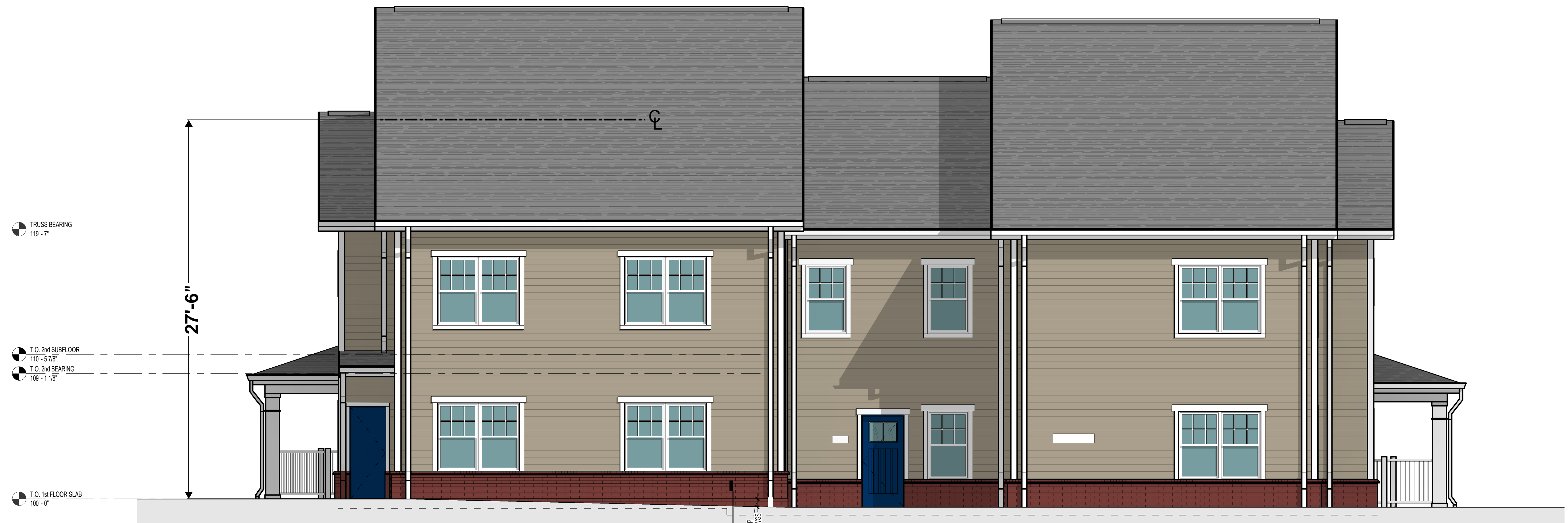
2 BLDG B #5 - STEPPED REAR ELEVATION 1/4" = 1'-0"
