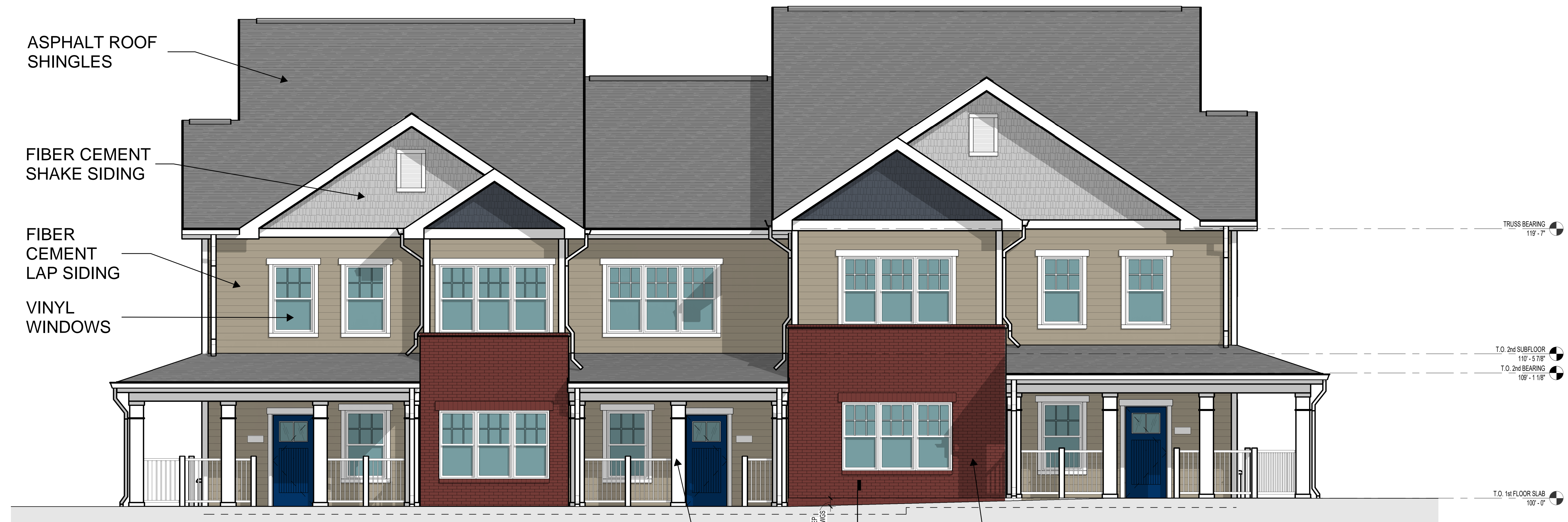
1 BLDG B #5 - STEPPED FRONT ELEVATION 1/4" = 1'-0"
