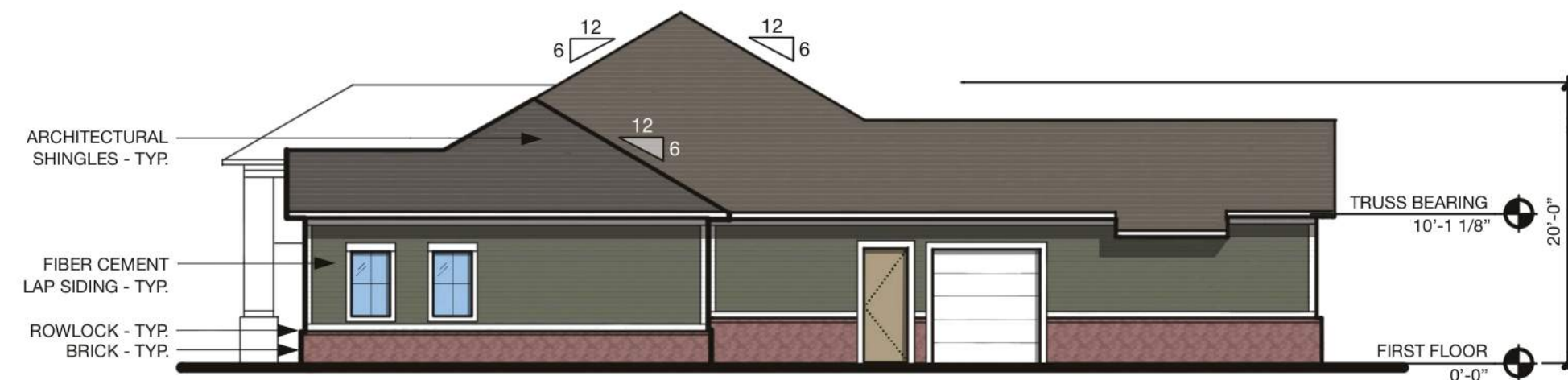
SIDE ELEVATION - COMM. BUILDING 3/32"=1'-0" B2
