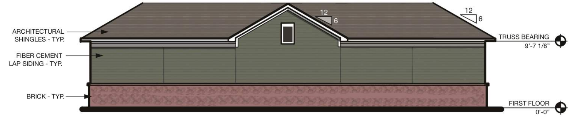
REAR ELEVATION - GARAGE 1/8"=1'-0" D1
