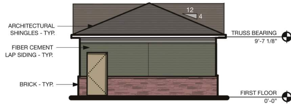
SIDE ELEVATION - GARAGE 1/8"=1'-0" D2
