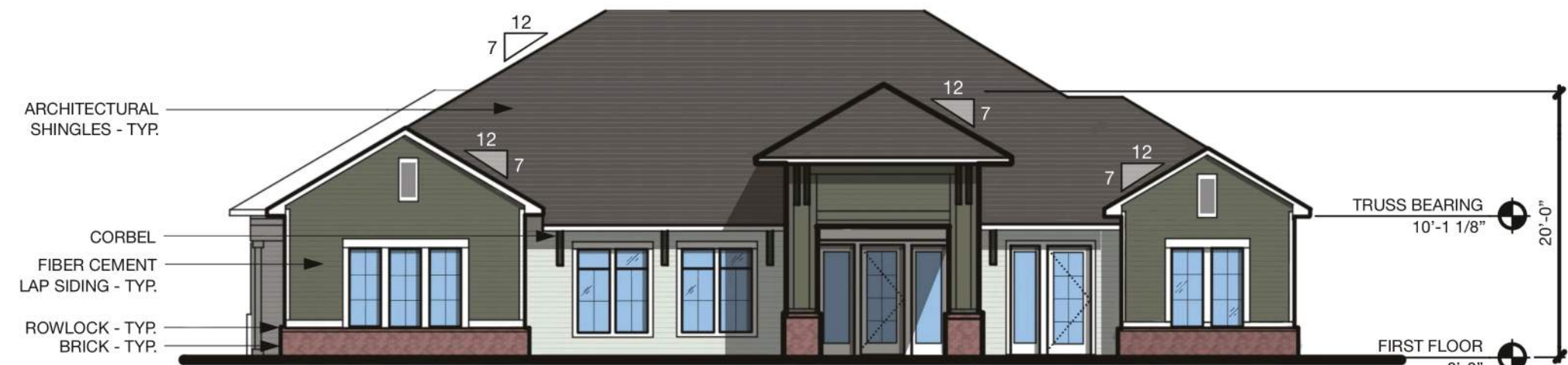
FRONT ELEVATION - COMM. BUILDING 3/32"=1'-0" A1
