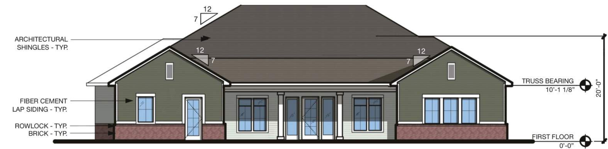
REAR ELEVATION - COMM. BUILDING 3/32"=1'-0" B1
