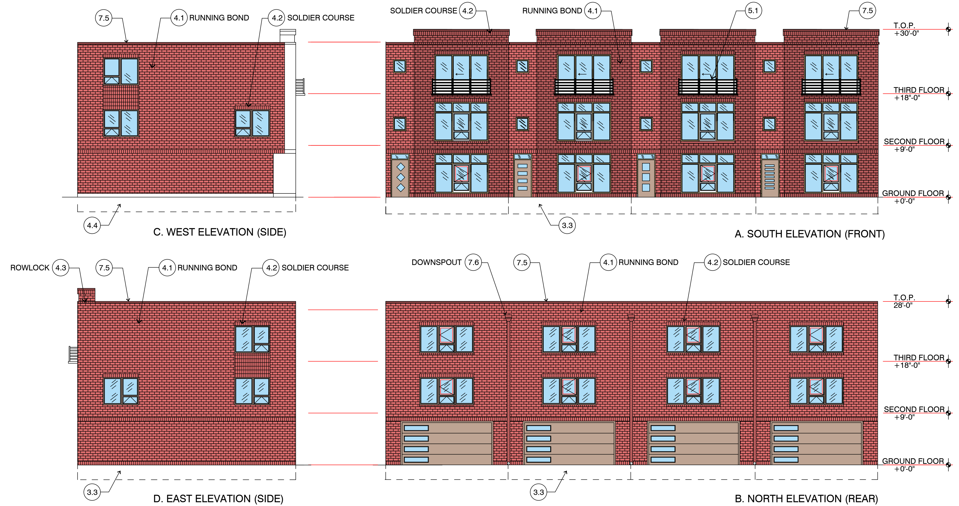
1 TYPICAL 4-PLEX BUILDING ELEVATIONS SCALE: 1/8" = 1'-0"
