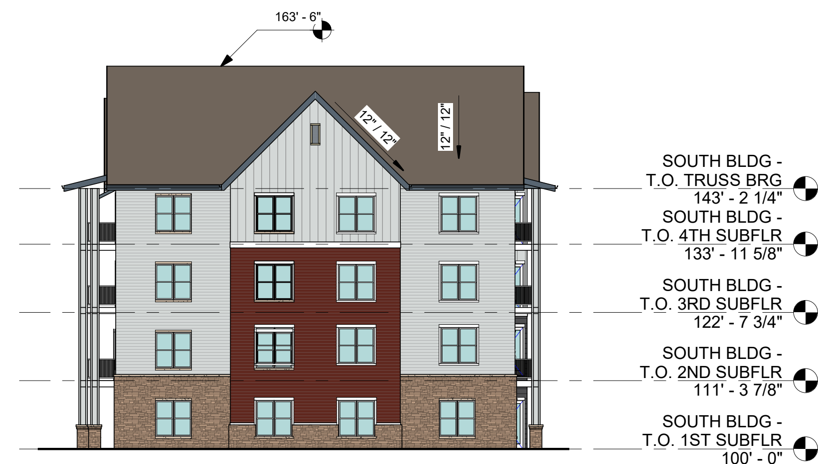
4 SOUTH BUILDING - WEST ELEVATION 1/16" = 1'-0"
