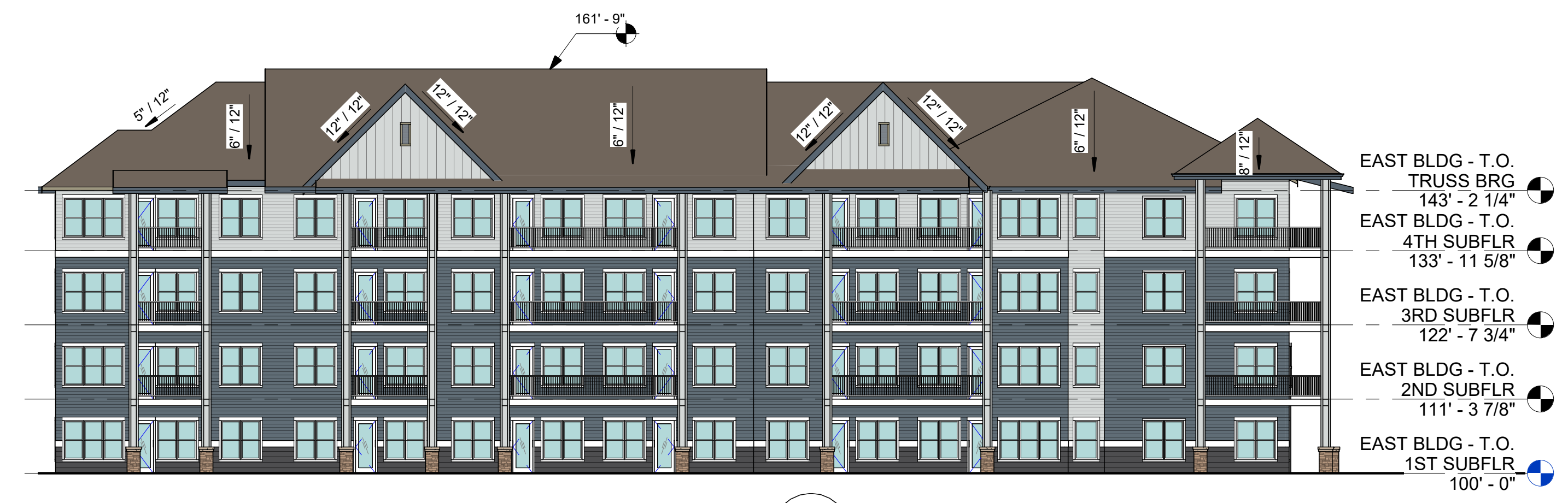
3 EAST BUILDING - EAST ELEVATION 1/16" = 1'-0"
