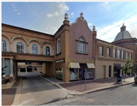
Example 1: Retail entrances on primary façade with direct access to sidewalk. Secondary entrances and service access are less prominent or visible from the sidewalk.
