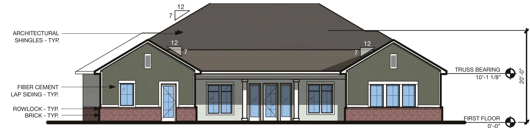
REAR ELEVATION - COMM. BUILDING 3/32"=1'-0" B1
