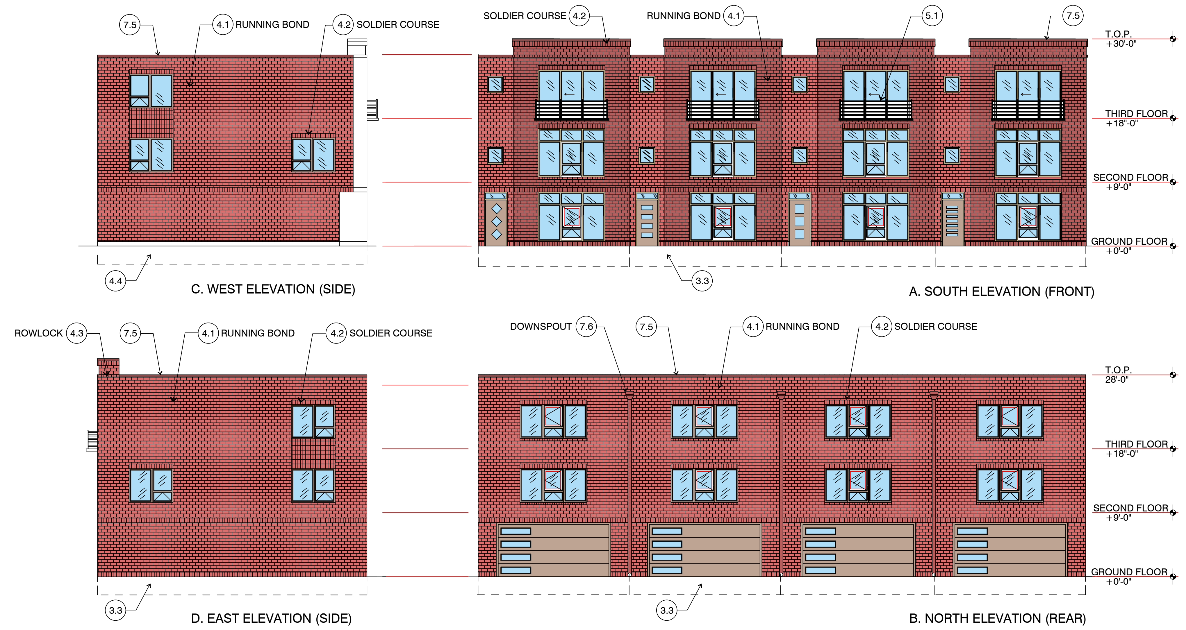
1 TYPICAL 4-PLEX BUILDING ELEVATIONS SCALE: 1/8" = 1'-0"
