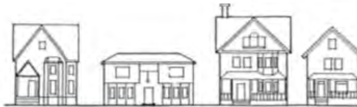
The patterns found along this street are not reflected in the second house. Unlike the other houses, this house has disproportionate windows, no porch, a low hip roof, and sits low to the ground.
