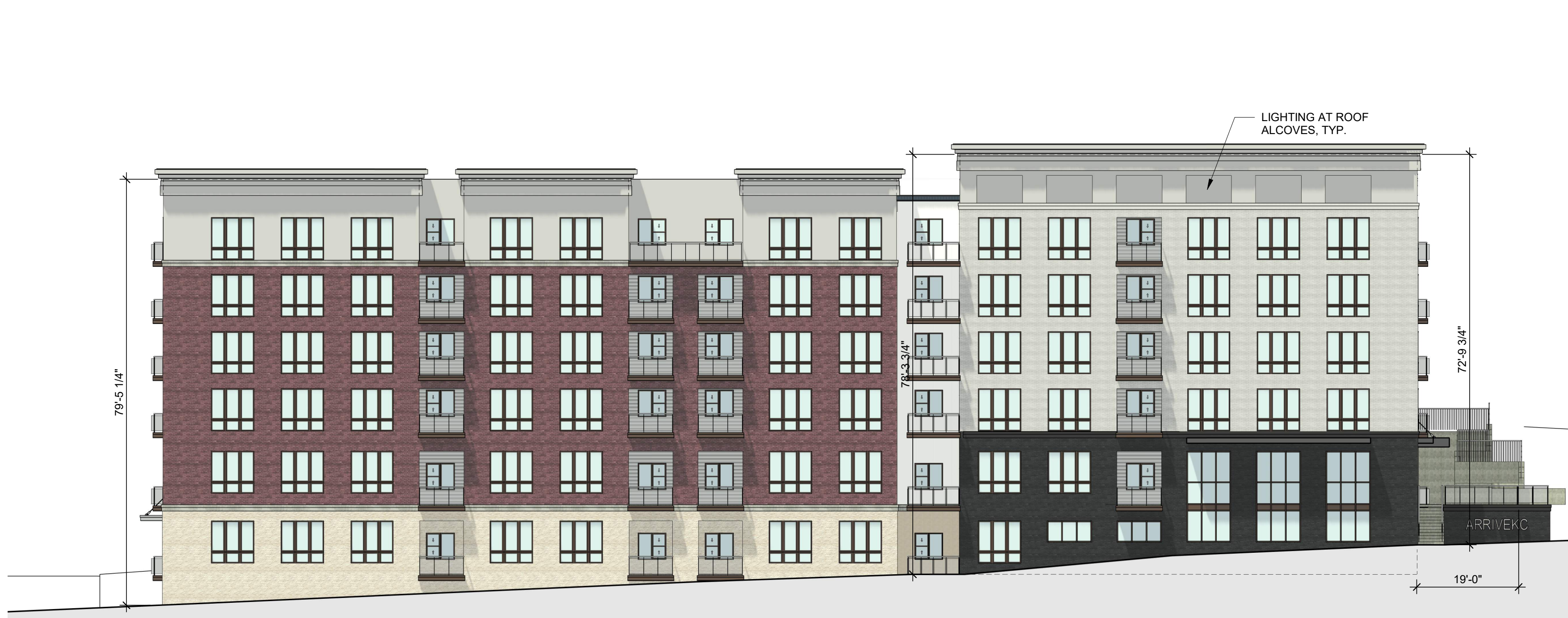
3 EXTERIOR ELEVATION 31st St. 1/16" = 1'-0"
