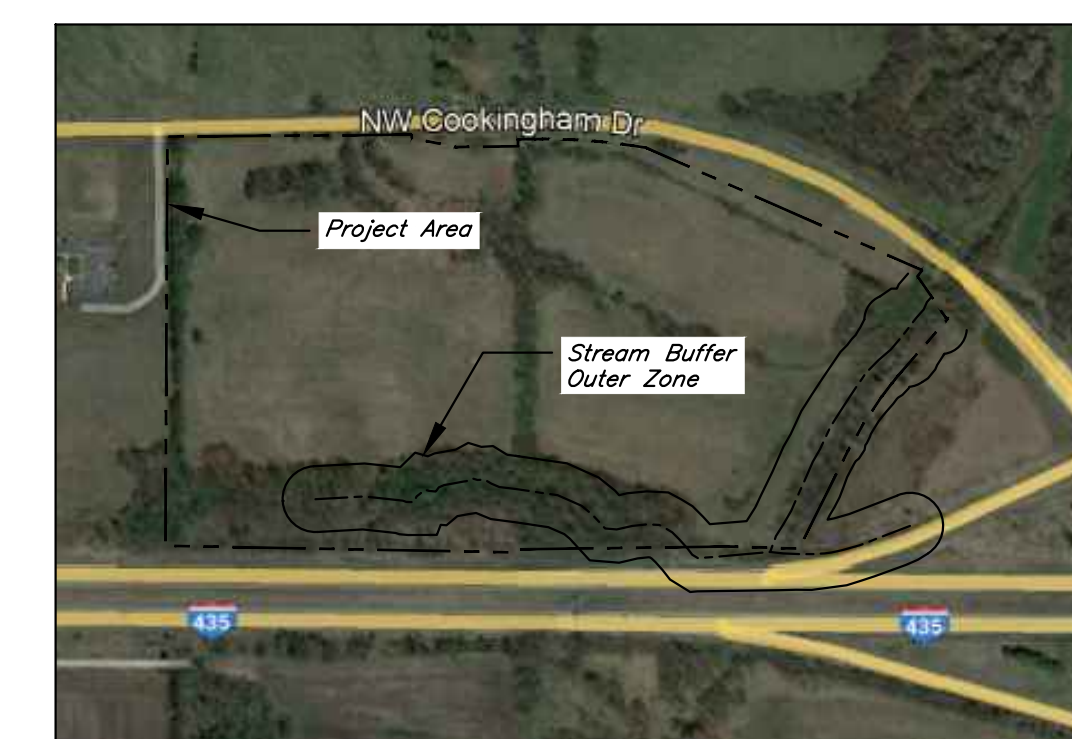
VICINITY MAP Not to Scale KCMO Regulated Stream within Property Boundary: Length = 2426 FT
