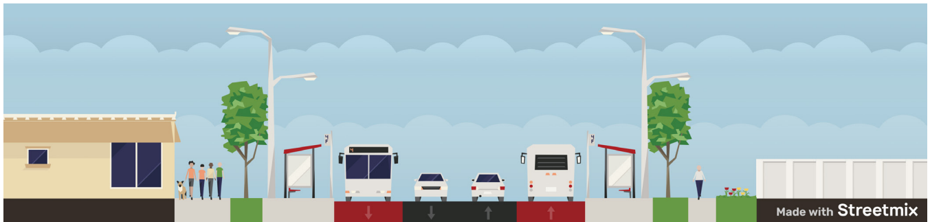
100-foot ROW: Two-way segment with transit-only lane on both sides
