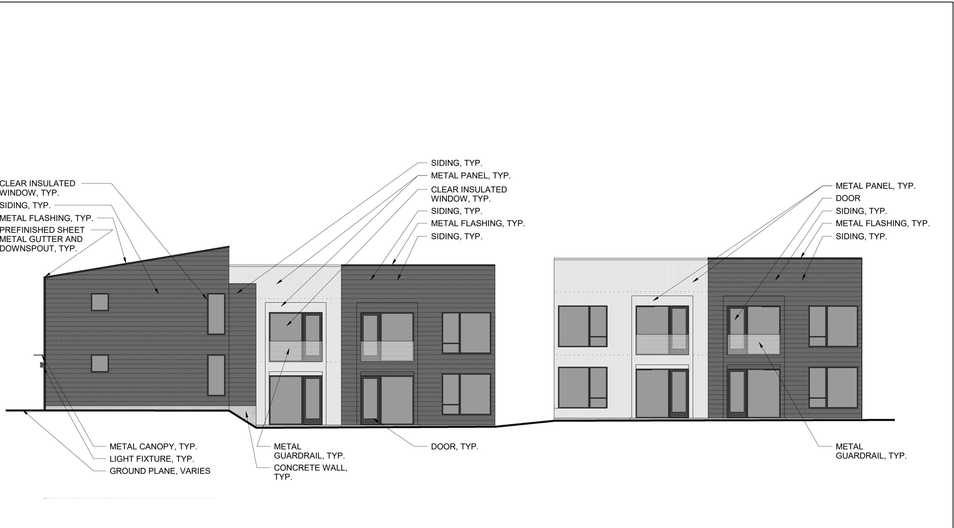
SOUTH ELEVATION E01 1/8" = 1'-0" 0' 4' 8' 16' 32'
