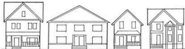
Although the second house reflects alignment in the placement of the windows, entry, cornice and roof, its proportions are not appropriate. Note the large horizontal windows, the double doors, and the overall width of the house.
