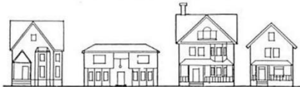
The patterns found along this street are not reflected in the second house. Unlike the other houses, this house has disproportionate windows, no porch, a low hip roof, and sits low to the ground.
