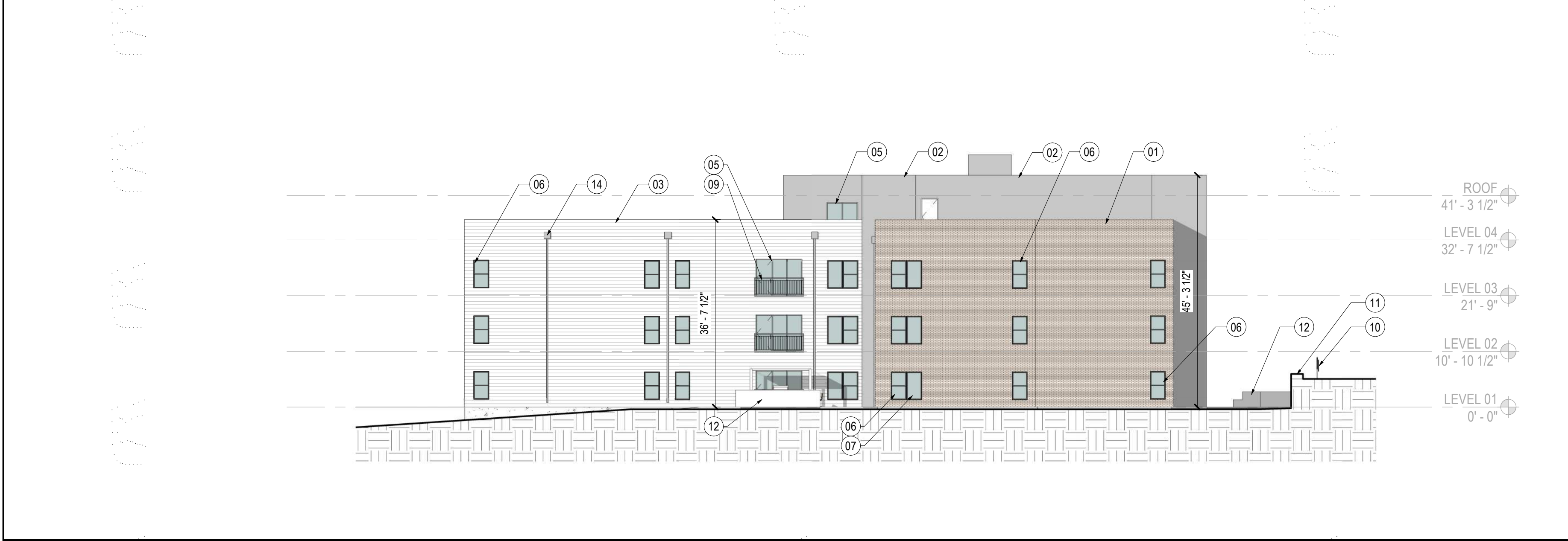
D08 SOUTH ELEVATION RE: A06 / A001 1/16" = 1'-0" 0' 2' 4' 6' 8' 10' 12' 14' 16' 18' 20' 22' 24' 26' 28' 30' 32'
