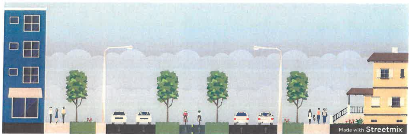
150-foot ROW: Two-way segment with wide median and two-way mobility lanes in the median
