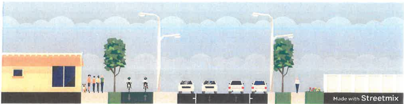
100-foot ROW: Two-way segment with parking lane on both sides and separated two-way mobility lanes
