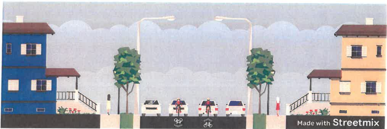
50-foot ROW: Two-way segment with shared lanes and parking permitted on both sides
