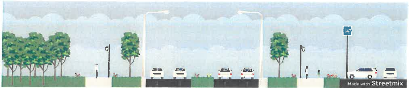
120-foot ROW: Two-way segment with median
