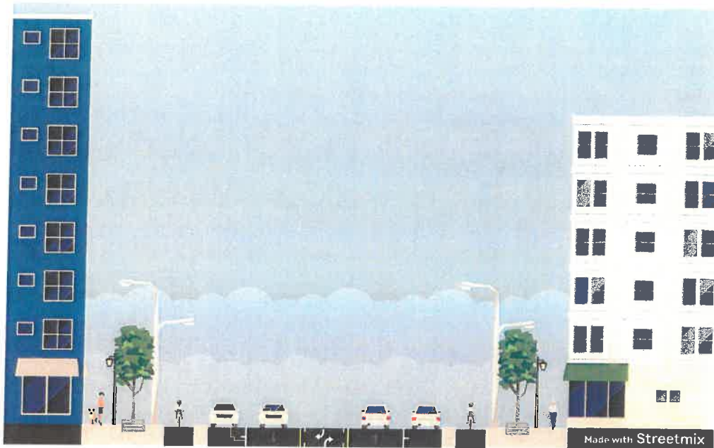
80-foot ROW: Two-way segment with center turn lane, parking lanes, and separated mobility lane on both sides
