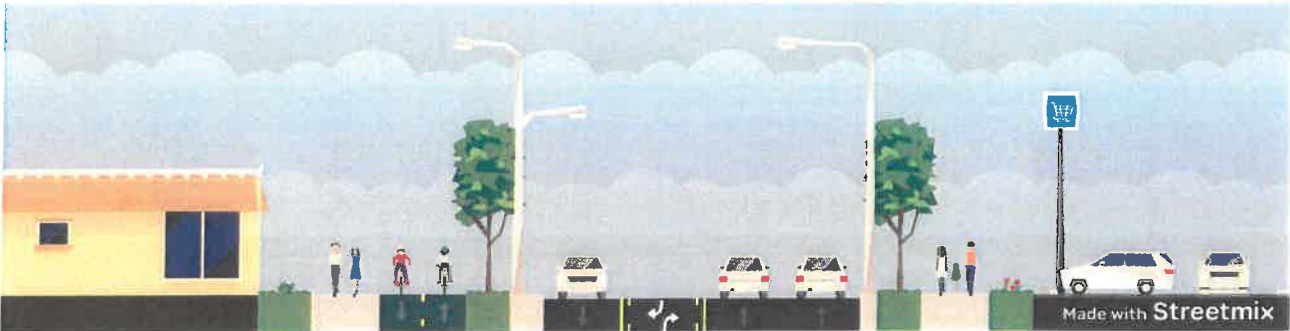
120-foot ROW: Two-way segment with center turn lane and separated two-way mobility lanes
