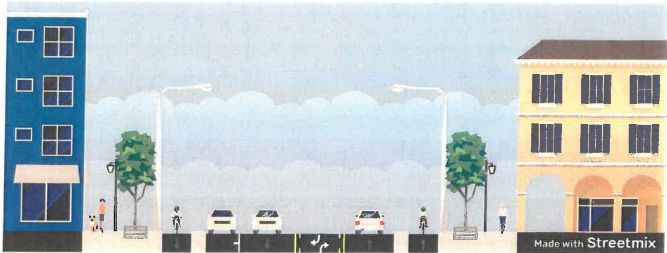
80-foot ROW: Two-way segment with center turn lane, parking lane on one side, and separated mobility lane on both sides
