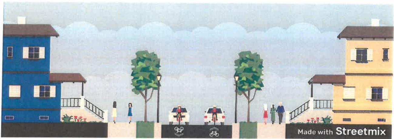
50-foot ROW: Two-way segment with shared lanes
