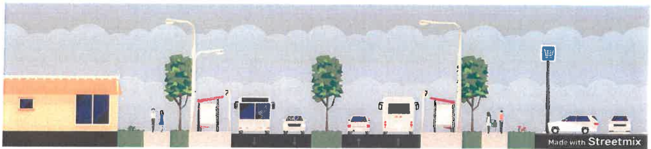
120-foot ROW: Two-way segment with median and transit facilities on both sides
