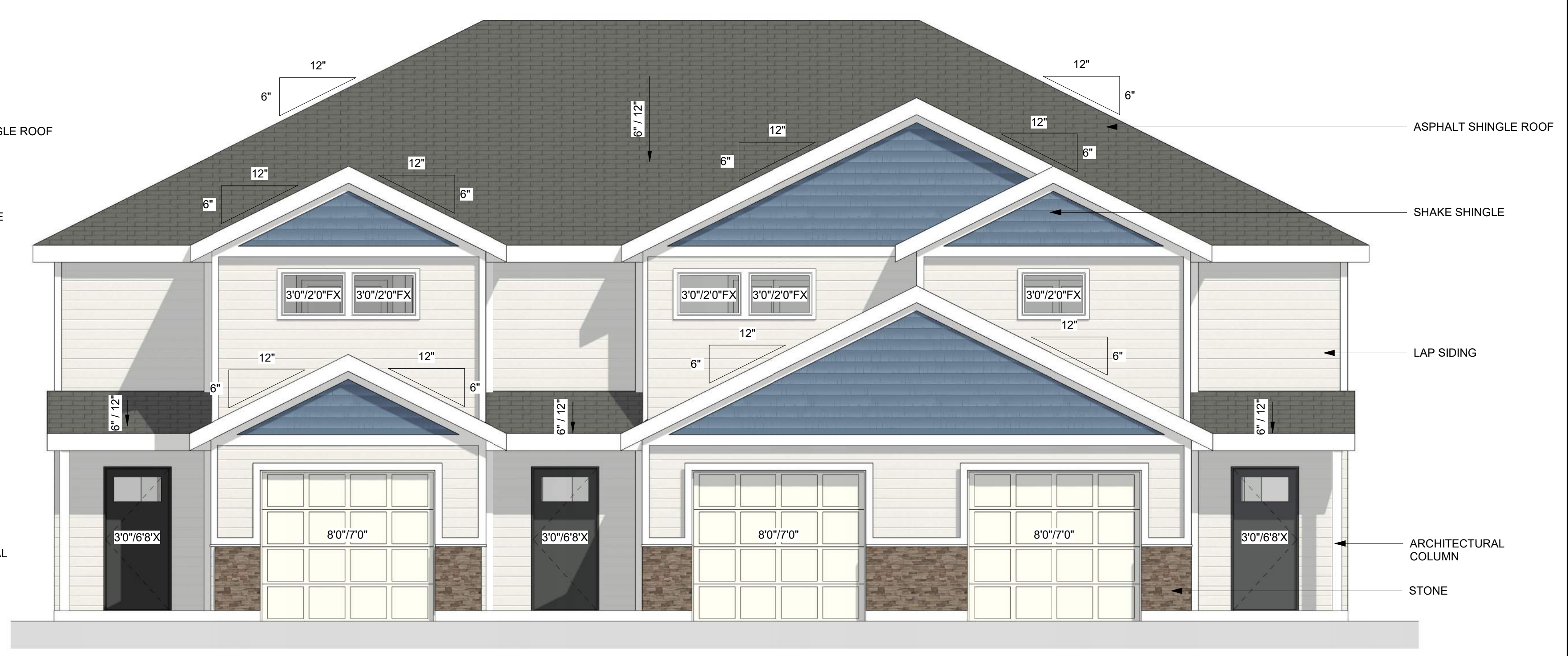
③ A2 TRIPLEX FRONT ELEVATION 1/4" = 1'-0"
