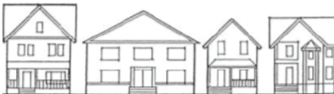
Although the second house reflects alignment in the placement of the windows, entry, cornice and roof, its proportions are not appropriate. Note the large horizontal windows, the double doors, and the overall width of the house.
