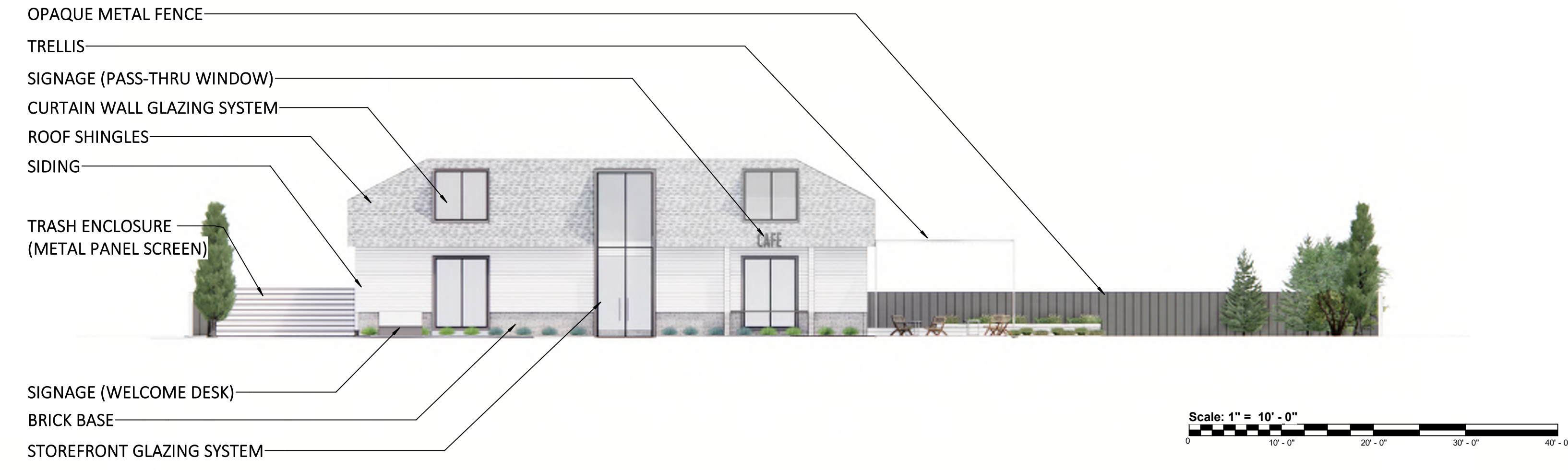
SOUTH ELEVATION_SUPPORT BLDG. L10 1" = 10'-0"
