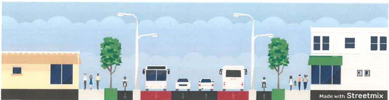
100-foot ROW: Two-way segment with transit-only lane on both sides and separated mobility lane on both sides
