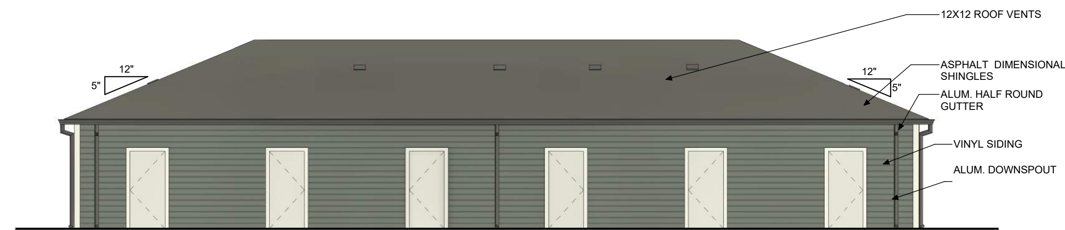
2 6-BAY GARAGE A - REAR ELEVATION 1/8" = 1'-0"
