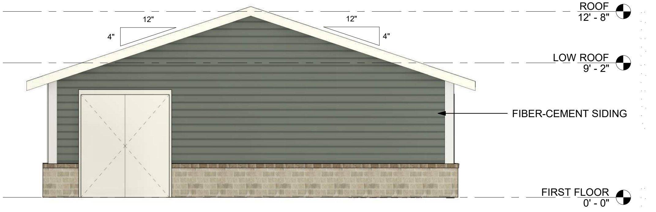
5 MAINTENANCE BUILDING - REAR ELEVATION 1/4" = 1'-0"
