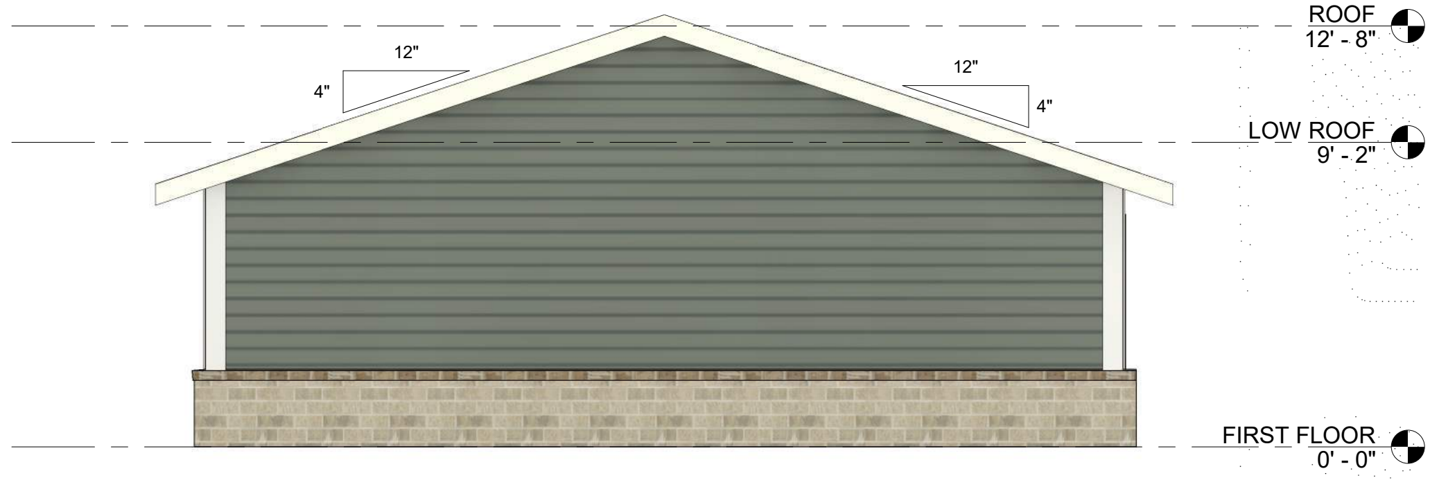
4 MAINTENANCE BUILDING - FRONT ELEVATION 1/4" = 1'-0"
