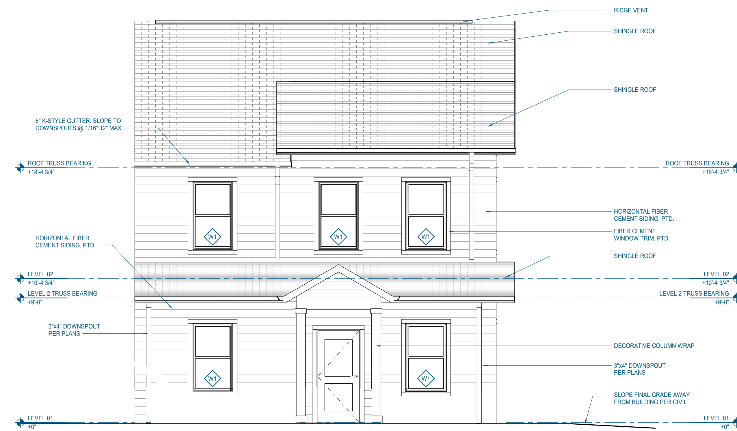
A09 H2* - FRONT ELEVATION 1/4" = 1'-0" | A-167
