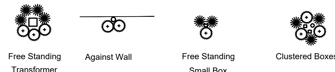
TYPICAL UTILITY BOX SCREENING DETAILS - NTS
